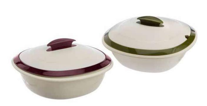
Comprising of an inner bowl, an outer bowl and an insulated server, the extra space on the bowl rim of this casserole helps easy placing and removal. The doubled walled insulation is achieved by nesting the two bowls of different sizes together, thus creating an air gap between the walls. The cover too, is double walled. Maximum heat is retained when the server is full. This casserole in fact provides you with two bowls to serve both hot and cold food.
